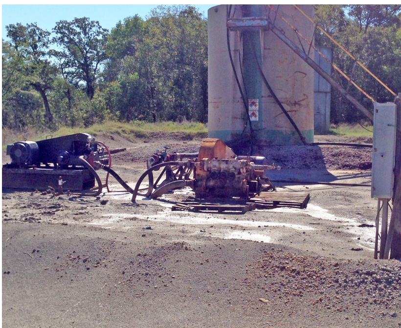
Hydra-Cell T8045 seal-less, leak-free triplex pump (left) replaced the leak-prone conventional triplex plunger pump on this injection well application in Texas.
